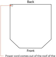
Power cord comes out of the roof of the sauna and is approximately 8 ft long.
