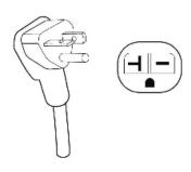
240V / 20 Amps Electrical Circuit Required NEMA 6-20p
