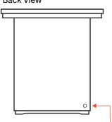
Power cord is located on the back of the sauna, six inches off the ground and is approximately six feet long.
